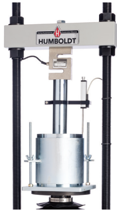
Figure #2 CBR Instrumentation Setup
