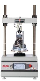
Semi-Circular Bending setup shown on HM-5030
