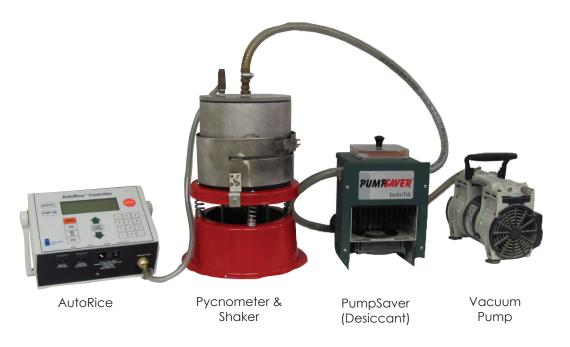
Fig 1. Maximum specific gravity (Rice) test equipment configuration
