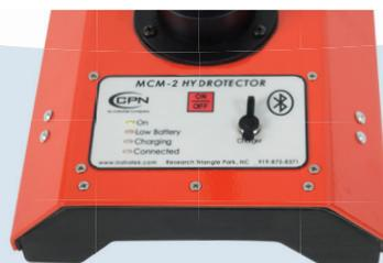
The Sensor keypad has one key – ON/OFF, four status LEDs, and the charger jack. 12V AC-DC charger provided.
