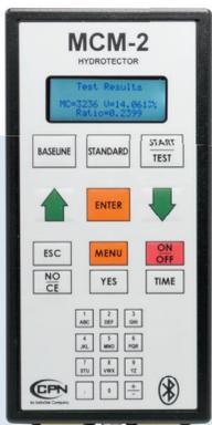
The Handheld control unit communicates with the sensor head using Bluetooth technology to collect data.
