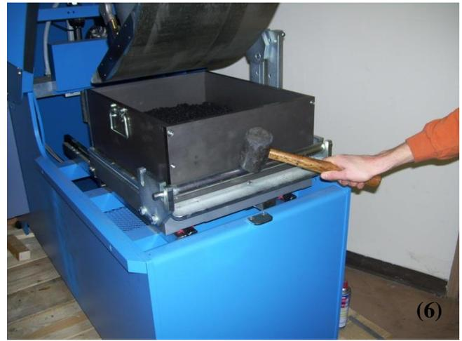
**Preparing mixture in mold to compact slab: (1)/(2) Scoop material evenly into heated mold, (3) Use multiple layers to ensure even density, (4) spread mixture evenly to improve density, (5) place mold in ARC, (6) lock mold into place with rubber mallet.**
