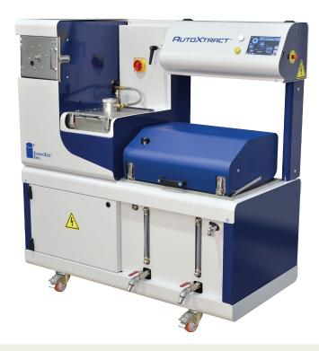
The AutoXtract™ is an innovative device that automates the processes associated with asphalt extraction and recovery. The unit has been designed for determination of asphalt content in mixtures as well as characterization of reclaimed asphalt pavement (RAP) properties.
