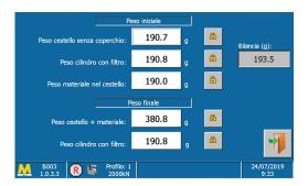
Automatic asphalt content calculation at the end of the test. Test results export to a .txt file to create customized reports.
