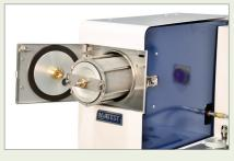
Mesh drum easily fits into washing chamber. Inspection window allows for monitoring of the solvent level.
