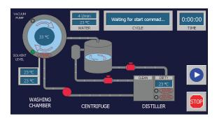
Test can be easily programmed. All phases and parameters can be monitored and changed in real time through the smart interface.
