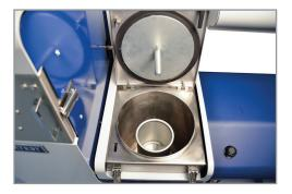
High speed centrifuge. Inspection window on the cover is used to monitor the solvent color during extraction.
