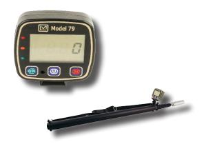
The Model 79/2 has three modes of operation - RATE, MAX, and COUNT. Measurements can be collected in two sets of units (primary and secondary) for RATE and MAX modes in cps, cpm, Sv/h, mrem/hr, and R/hr units. The user can choose by simply pressing the Units button. An internal switch is used to enable or disable the front-panel setup feature to protect desired settings from inadvertent modification. Setup is also available via software from Ludlum Measurements.
