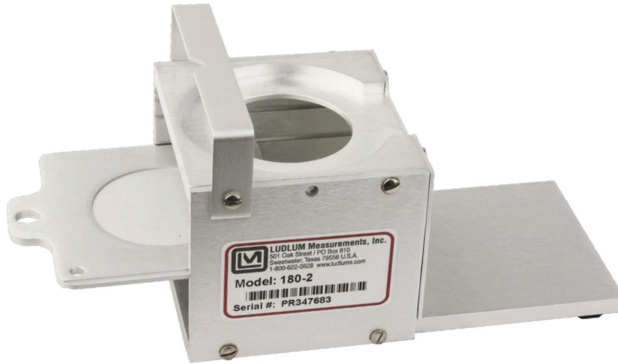
The Model 180 Series of sample holders are designed to ensure accuracy and repeatability when counting samples. This model has five levels for the sample tray and permits the user to select the desired distance by merely sliding the tray into the corresponding groove. A notch accommodates the handle of the commonly-used Model 44-9 Detector (below) to permit parallel positioning of testing sample and the detector face.
