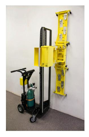
The above photo shows the gas proportional version (without cables) of the Model 240 (PN: 48-3956), in the wall monitoring position. Below is the Model 240S (PN: 48-4131), the scintillation version, shown in the floor monitoring position.
