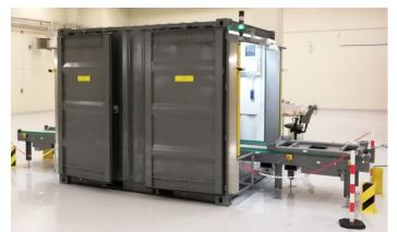
HWM-1800C in a 5-foot container incl. conveyors on the entrance and exit side (option)
