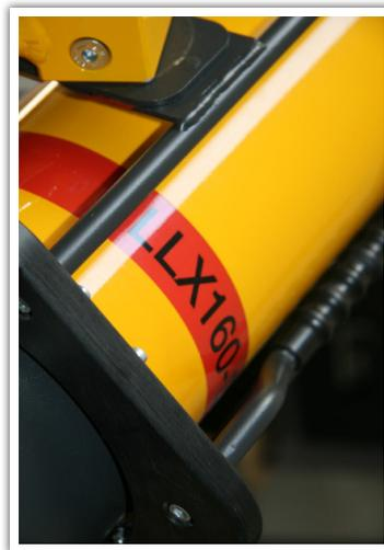
The LLX160-DA is a high frequency constant potential Directional Air cooled, portable X-ray generator that can be used in combination with digital detectors.
