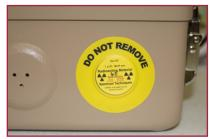
(left) Stick-On Check Source in Model 4464-473 Holder (right) Stick-On source applied in typical fashion to instrument case
