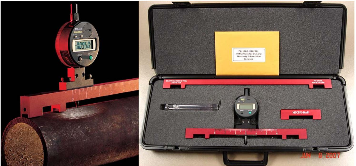
Profiles can be assessed quickly and accurately by sliding the digital gauge along the bridging bar. Notched feet and ceramic magnets prevent the bridge from rocking on the pipe. The magnets securely hold the bridge in place which makes it ideal when working upside down. Locking adjustment screws allows instant calibration to reference surface. Pointed and needle tips find the deepest section of pits with ease.
