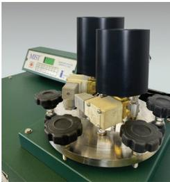
**InstronTek's MiST 2**, the best asphalt moisture sensitivity conditioning device, upgraded with an ultra-quiet pressure system and a small footprint to fit inside any size asphalt lab. MiST 2 test results can determine both the adhesive and cohesive properties of asphalt mixtures to help alleviate moisture issues in the field. The New & Upgraded MiST 2 is quieter, more compact and user-friendly with advanced features to make the system operate more efficiently.
