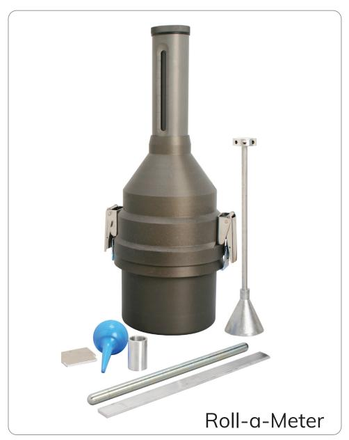
The following instructions are intended only as a guide for general operation of the meter. For complete and detailed test operating instructions, please refer to current ASTM C173/C 173M. C29/C29M and C172 specifications.
